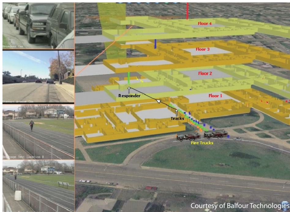
3D building model geo-located on a campus, aerial imagery with floor plans overlaid, and responders being tracked through the building.
